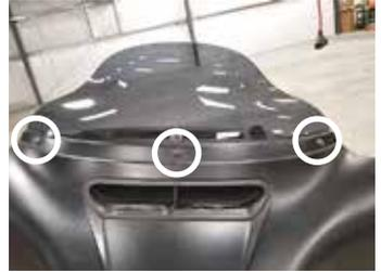
**TIP:** Reinstalling the center screw after removing the windshield will prevent the outer fairing from falling during the next step. A few turns by hand will be sufficient.
